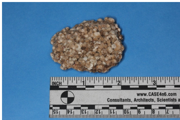
Figure 44. Solidified Fertilizer Collected from WFC Property (Approximate Location Unknown) (Source: Forensic Laboratory)
