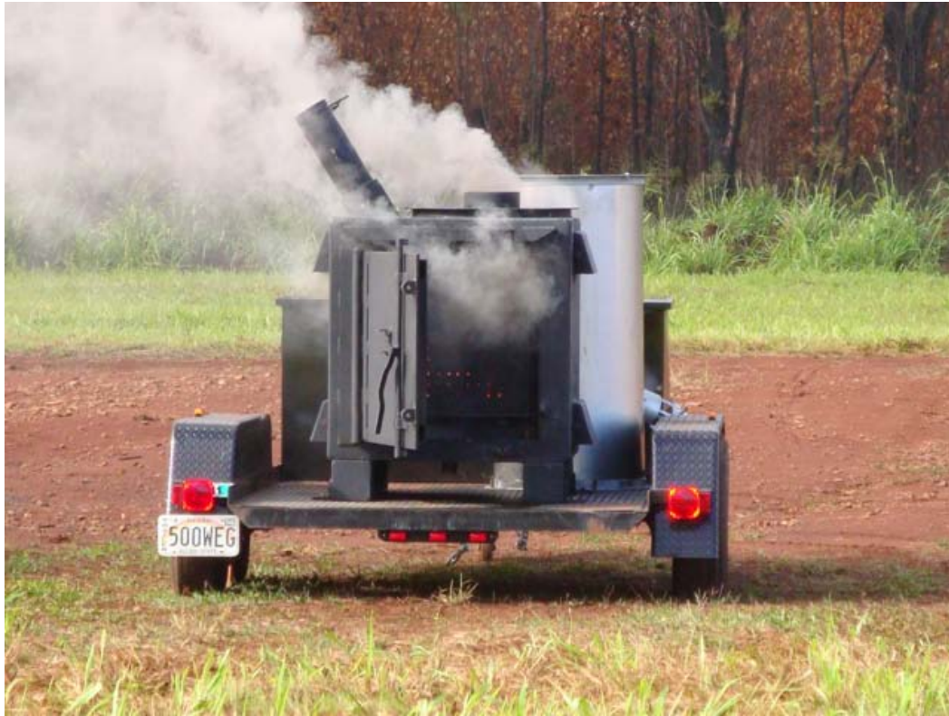
Figure 10. Fireworks burning in incinerator (TFU)
