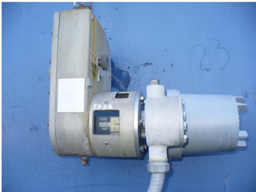
Figure 4: Side gauge: mounted on the side on a tank and displaying the amount of liquid in the tank
