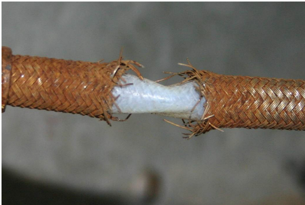
Figure 15. Damaged hillside phosgene hose removed from phosgene cylinder. The plastic adhesive tag that covered the damaged section fell off during the hose decontamination procedure.
