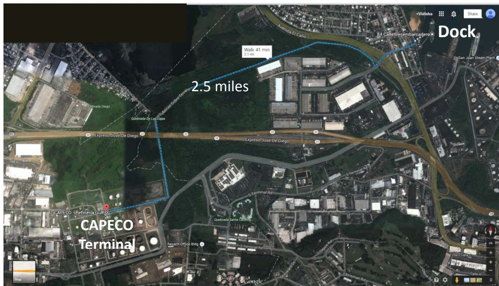
Figure 2: CAPECO Pipeline to Gulf Oil Dock where gasoline is offloaded from ships
