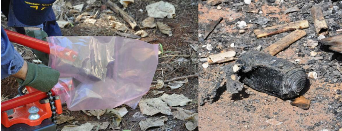
Figure 22. Left photo (courtesy of ATF) shows anti-static bag used by ATF post-incident; right photo shows a roll of plastic garbage bags found following the incident.
